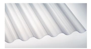
SmartPIU is an innovative 2.5 mm thick multiwall corrugated polycarbonate sheet for use in domestic and home improvement roofing applications. The uniqueness of this product lies in its strength, spans and clean appearance. Product spans up to 1500mm separate SmartPIU from all other polycarbonate seen on the market today.
