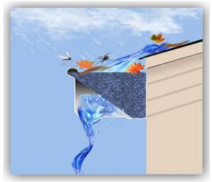
Gutter Protector sits inside the gutter so is invisible from ground level
