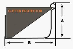
Gutter Protector will not clog, as the cell structure size of the product has been design to allow dust and silt to wash through into your gutter.
